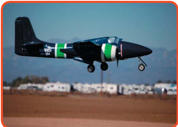
Denny Mallot's 80" Hobby People F7F Tigercat on an approach. Powered with two AXI 4130 brushless motors.
