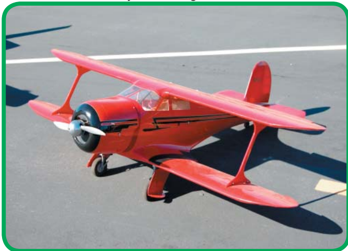
Robert Stanley's Top Flite 72" Beech Staggerwing with a ton of scale upgrades. Powered with an Enya V-240 four stroke.
