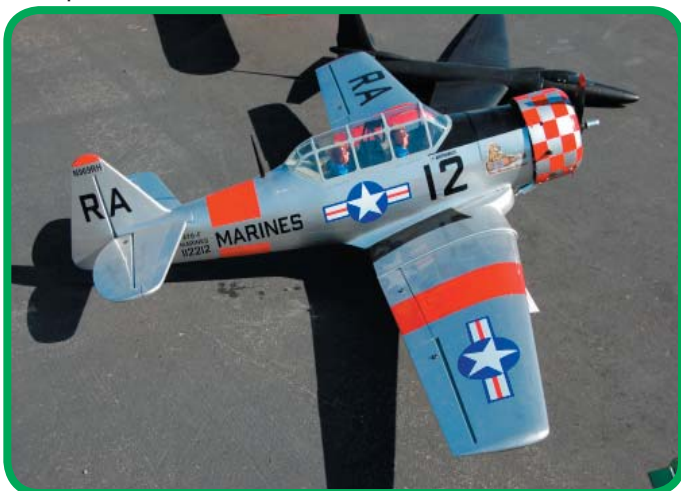
This is a new BH Models T6 from Hobby People with a 91 magnum four stroke for power. Great flyer and includes the retracts. Flown by Sam Wright.
