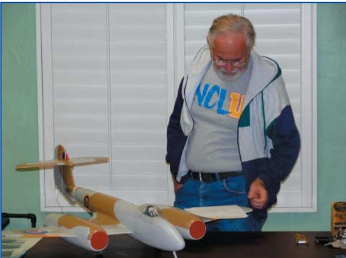
Master Builder Richard Burman shows his all scratch built Glouster Meteor. The meteor is a twin electric ducted fan model.
